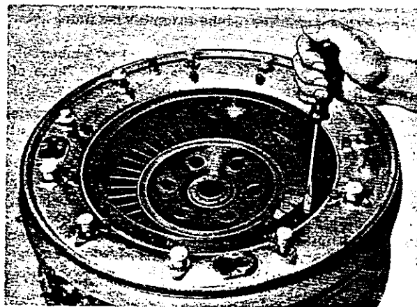
Figure 4-4. Installing Power Turbine Nozzle to Combustion Chamber Screws
